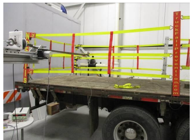
Photograph 84: Side Rear Middle Middle Strap Outboard Pull Setup (3)
