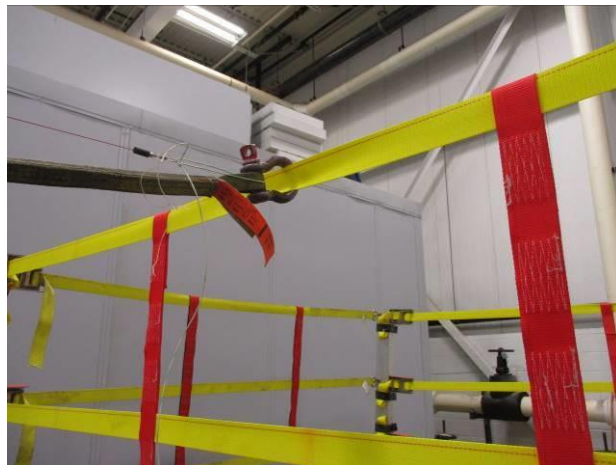
Photograph 98: Side Rear Middle Top Strap Outboard Pull Setup (2)
