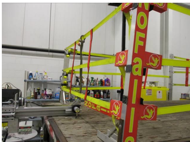
Photograph 21: Rear Top Strap 90 Degree Pull Setup (4)
