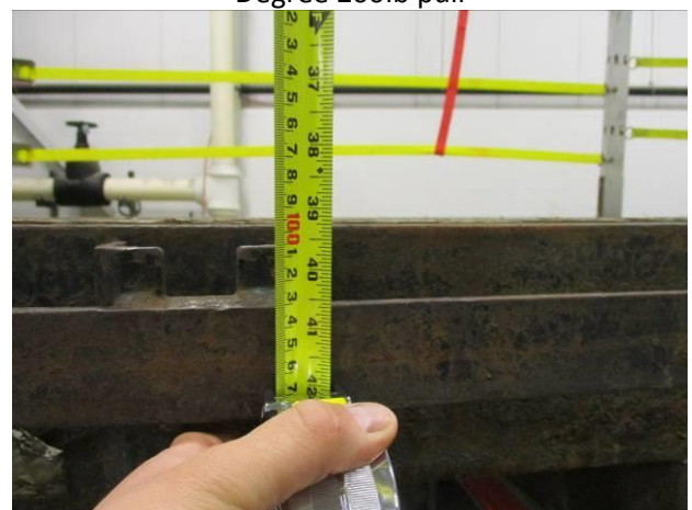
Photograph 96: Side Rear Middle Top Strap Height at 70 Degree Pull
