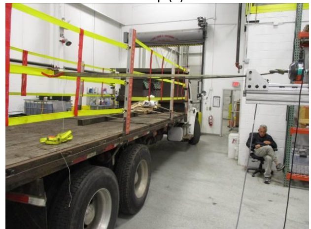
Photograph 82: Side Rear Middle Middle Strap Outboard Pull Setup (1)
