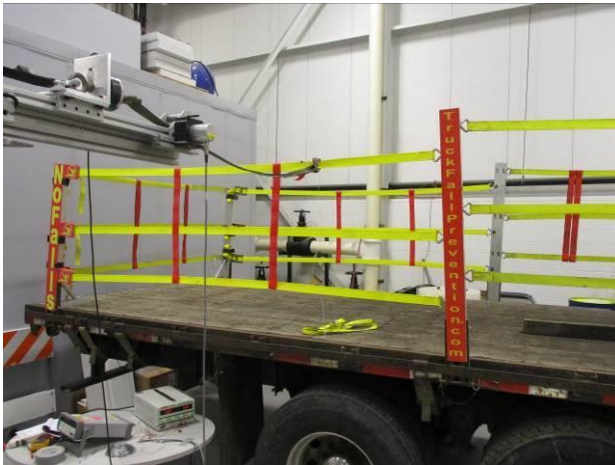
Photograph 79: Side Rear Front Top Strap Outboard Pull Setup (4)
