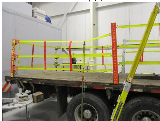
Photograph 76: Side Rear Front Top Strap during Downward Pull
