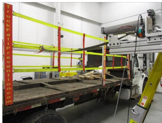
Photograph 62: Side Middle Rear Middle Strap Outboard Pull Setup (1)
