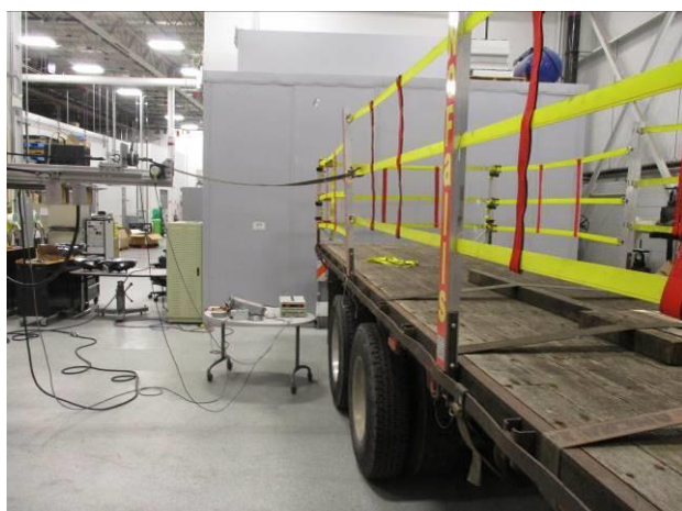
Photograph 65: Side Middle Rear Middle Strap Outboard Pull Setup (4)
