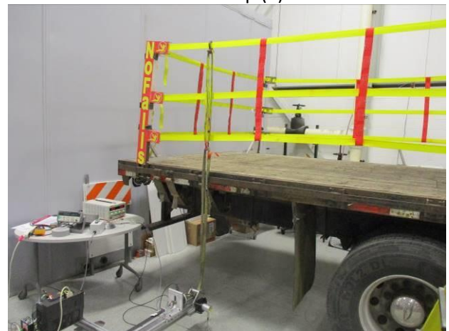
Photograph 108: Side Rear Rear Top Strap Downward Pull Setup
