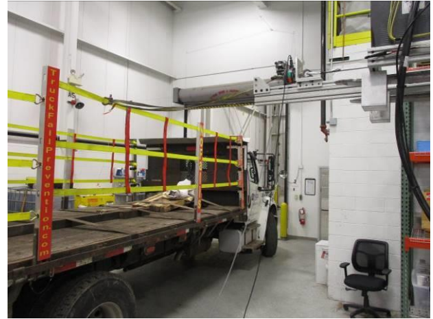
Photograph 68: Side Middle Rear Top Strap Outboard Pull Setup (1)
