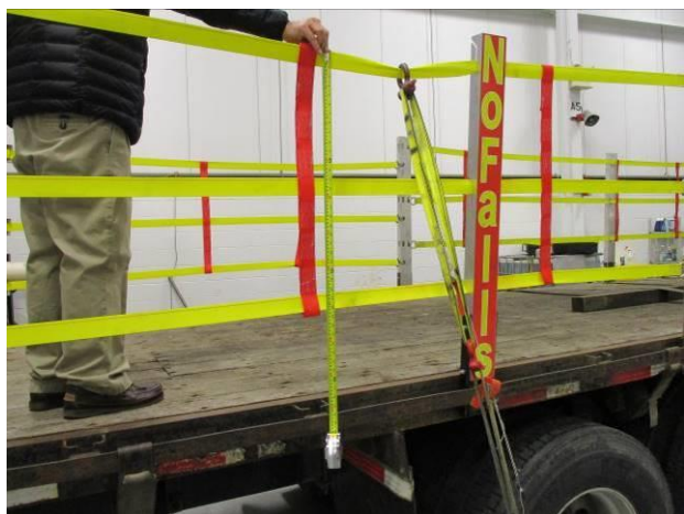
Photograph 89: Side Rear Middle Top Strap 70 degree Pull with Extra Post
