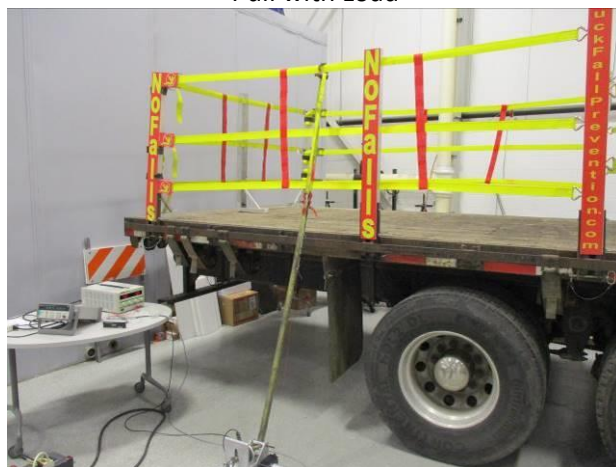
Photograph 88: Side Rear Middle Top Strap 70 degree Pull with Extra Post (2)
