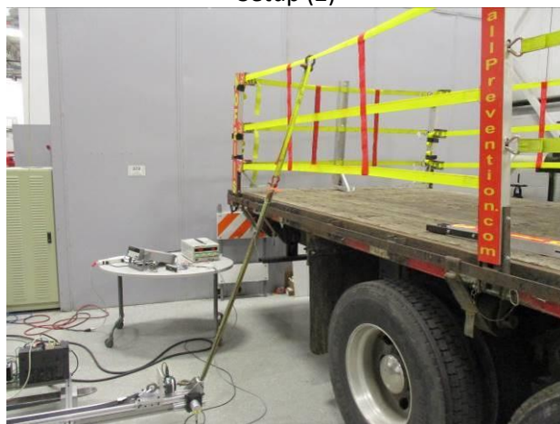
Photograph 100: Side Rear Middle Top Strap Pull at 70 Degrees (1)
