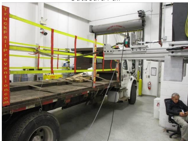
Photograph 63: Side Middle Rear Middle Strap Outboard Pull Setup (2)
