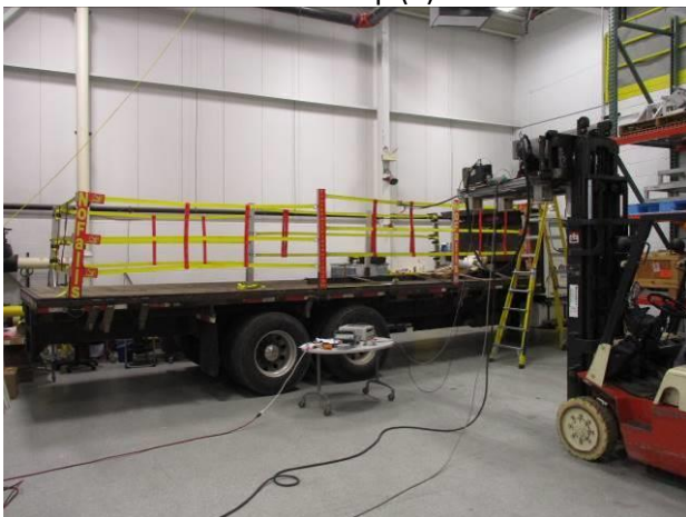
Photograph 59: Side Middle Middle Top Strap Outboard Pull Setup (3)
