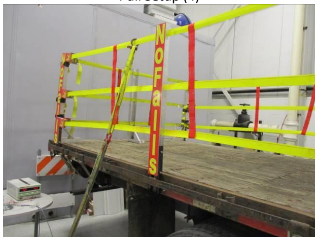
Photograph 87: Side Rear Middle Top Strap 70 degree Pull with Extra Post (1)
