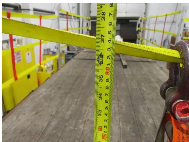
Photograph 23: Rear Top Strap Height during 90 Degree Pull
