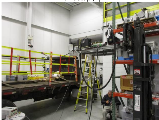
Photograph 51: Side Middle Front Top Strap Outboard Pull Setup (1)
