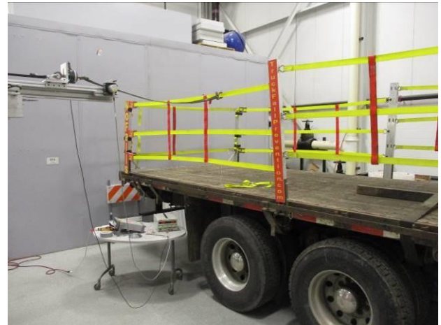
Photograph 80: Side Rear Front Top Strap Outboard Pull Setup (5)
