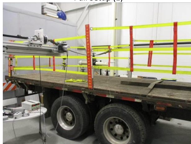
Photograph 64: Side Middle Rear Middle Strap Outboard Pull Setup (3)
