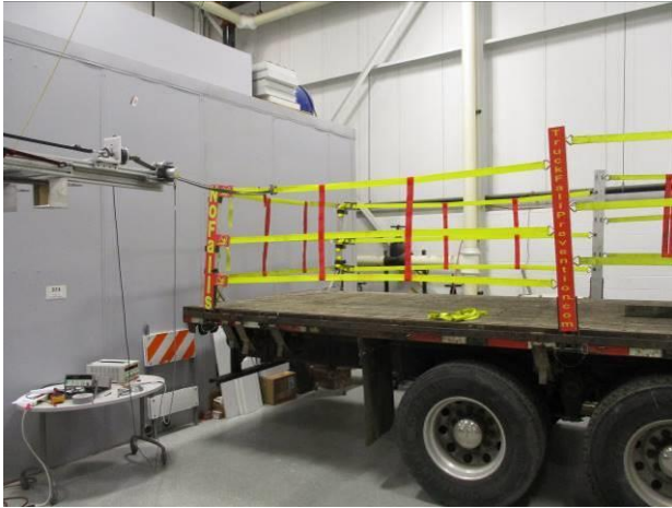
Photograph 109: Side Rear Rear Top Strap Outboard Pull Setup (1)
