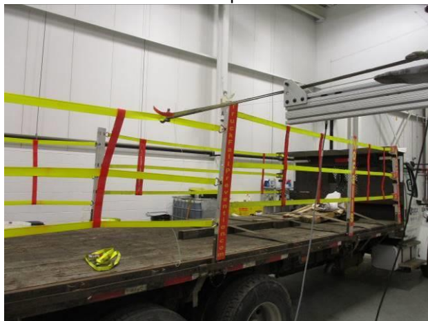
Photograph 77: Side Rear Front Top Strap Outboard Pull Setup (2)
