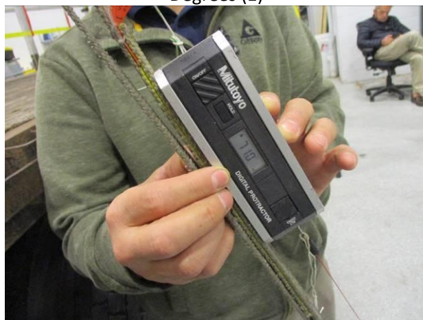
Photograph 102: Side Rear Middle Top Strap Pull at 70 Degrees (3)
