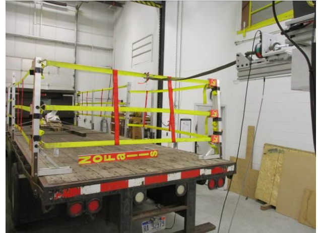
Photograph 26: Rear Top Strap Outboard Pull Setup (1)
