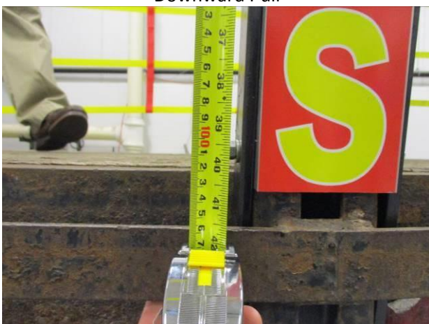
Photograph 95: Side Rear Middle Top Strap Height at 70 Degree Pull with Extra Post
