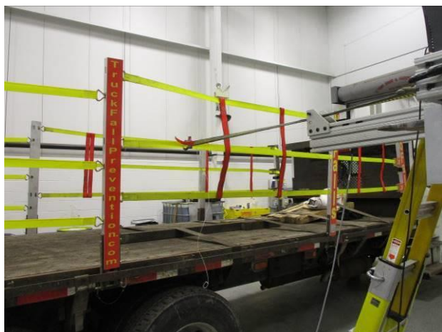
Photograph 61: Side Middle Rear Middle Strap during Outboard Pull
