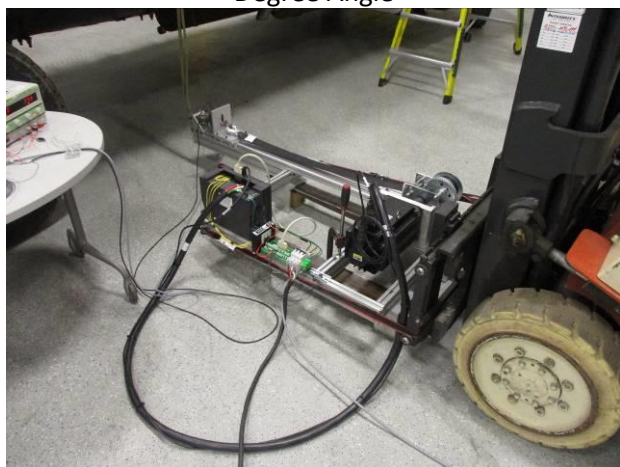
Photograph 45: Servo Pull Rig
