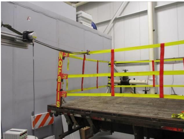
Photograph 111: Side Rear Rear Top Strap Outboard Pull Setup (5)
