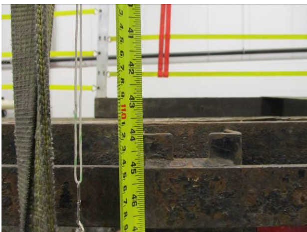
Photograph 5: Middle Rear Top Strap Height to Deck with 200lb Applied
