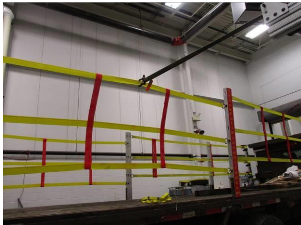
Photograph 97: Side Rear Middle Top Strap Outboard Pull Setup (1)
