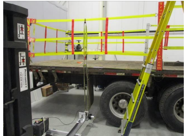
Photograph 92: Side Rear Middle Top Strap Downward Pull Setup (2)
