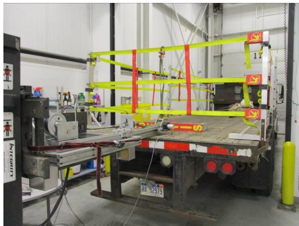
Photograph 20: Rear Top Strap 90 degree Pull Setup (3)
