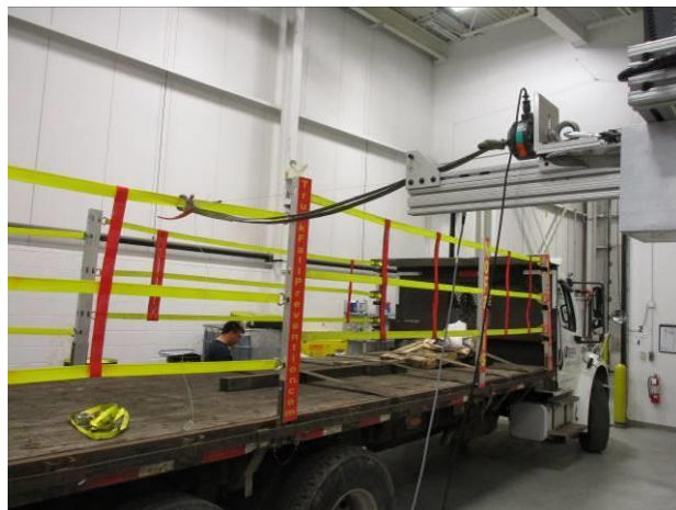
Photograph 78: Side Rear Front Top Strap Outboard Pull Setup (3)
