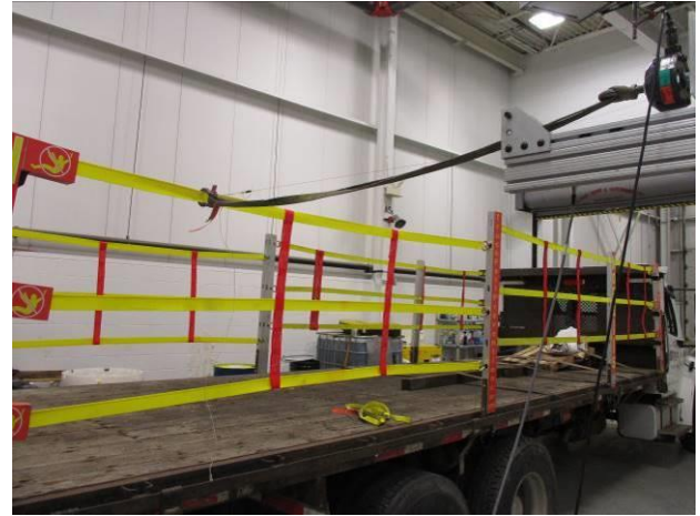
Photograph 110: Side Rear Rear Top Strap Outboard Pull Setup (4)
