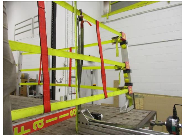
Photograph 18: Rear Top Strap 90degree Pull Setup (1)
