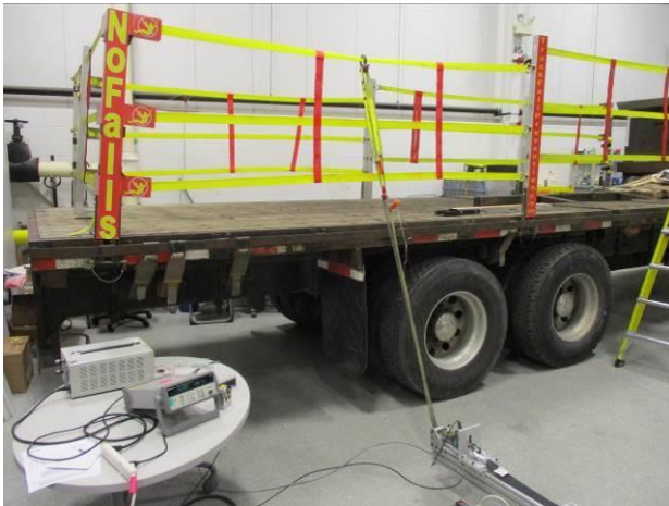
Photograph 103: Side Rear Middle Top Strap Pull at 70 Degrees (4)
