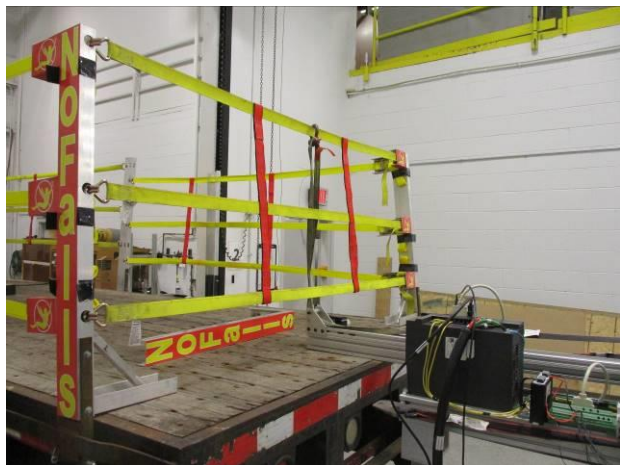
Photograph 19: Rear Top Strap 90 degree Pull Setup (2)
