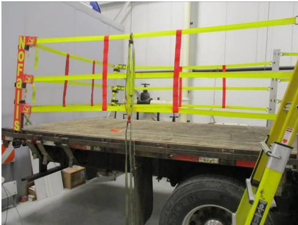
Photograph 91: Side Rear Middle Top Strap Downward Pull Setup (1)
