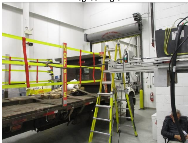
Photograph 46: Side Middle Front Middle Strap Outboard Pull Setup (1)
