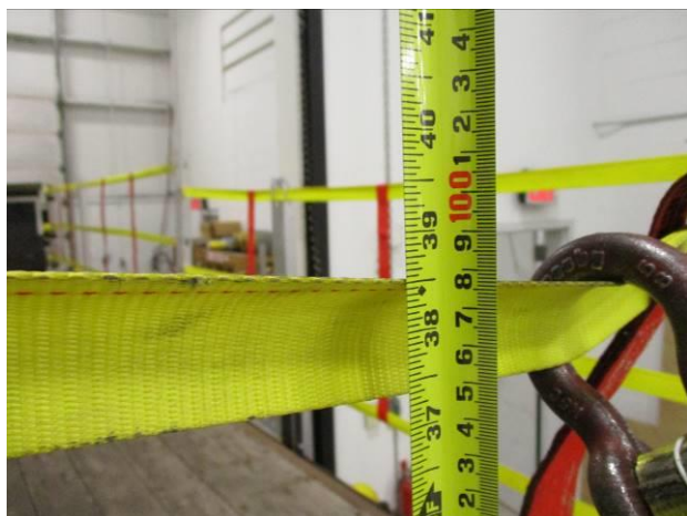
Photograph 43: Rear Top Strap with 200lb Applied at 50 Degree Angle
