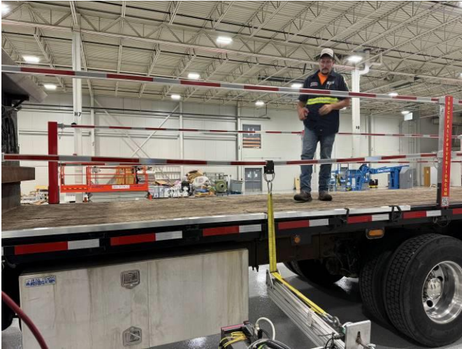
Figure 3: Midrail Under Load
